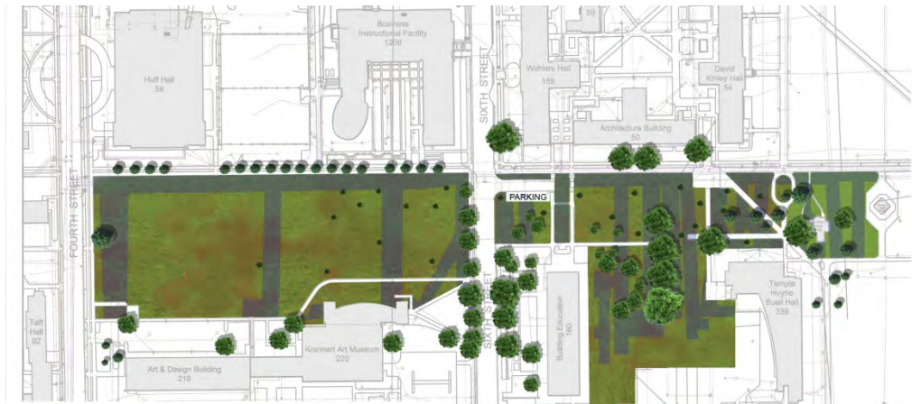
Figure 3. The grey areas indicate locations of under-ground utilities plus 15 ft. buffers around them.
